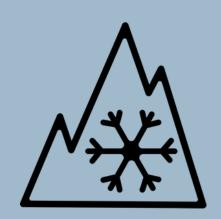
The 3PMSF marking confirms that a tire has passed strict tests for traction, braking and handling on snow and ice.
