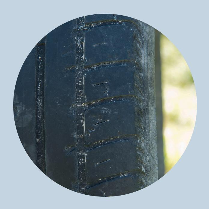
Use a tread depth gauge or the simple **coin test**, good for most on-the-road tires: Insert a €2 coin into the tread. If you see the silver rim, it's time to change!
